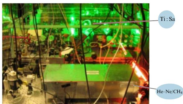
**Figure 4.** Stationary methane optical clock facility at JILA, Boulder, USA (2004). In the foreground is FIAN's He–Ne/CH<sub>4</sub> OFS. Ti:Sa is a Ti:Sapphire femtosecond laser.
