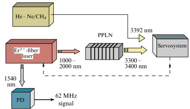
**Figure 2.** Schematic of a compact methane optical clock. PPLN is a crystal of periodically poled lithium niobate, and PD is a photodetector which records femtosecond laser pulses.
