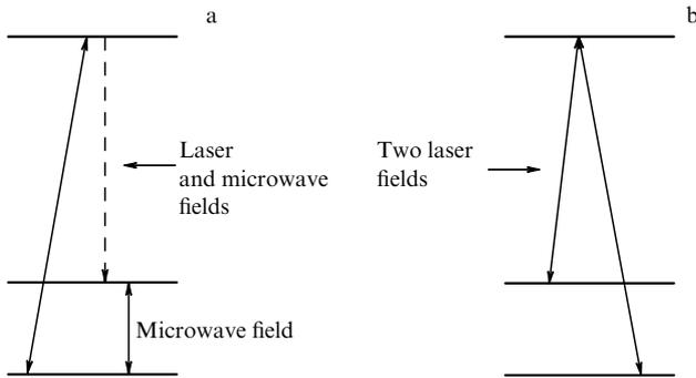
**Figure 1.** Traditional scheme (a) of a microwave standard and of the novel one, which makes use of coherent population trapping (CPT) resonance (b). In the case (a), atoms experience a microwave field and one optical field. The dashed line shows the spontaneous transition. In the case (b), the atoms are irradiated by two laser fields with a frequency difference determined by the microwave field.
