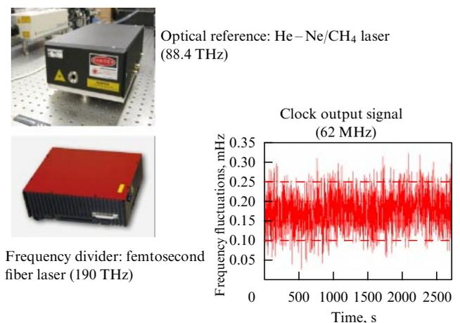
**Figure 3.** Main components of the compact optical clock and frequency-counter readings of the output signal (for an averaging time of 1 s). (The frequency counter is locked to a VCH-1006 hydrogen maser.)
