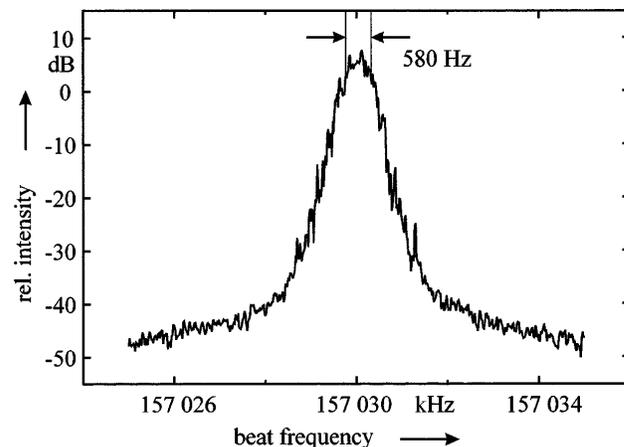
Fig. 3. Beat note between the DLS and a dye-laser spectrometer when the master laser is locked to the high- $Q$  cavity. Resolution bandwidth, 300 Hz; video bandwidth, 10 Hz; seep time, 10 s.
