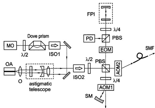
Fig. 1. Optical schematic of the experimental setup: MO, master oscillator; OA, optical amplifier; O, collimating objective; ISO1, ISO2, 40-dB optical isolators; SM, spherical mirror; PD, photodiode; PBS's, polarizing beam splitters; SMF, single-mode fiber delivering laser radiation to the magneto-optical trap. Other abbreviations defined in text.
