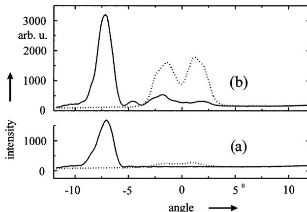
Fig. 2. Far-field distribution of the amplified output with (solid curves) and without (dotted curves) injected light from the master laser for amplifier currents of (a) 215 mA and (b) 250 mA.
