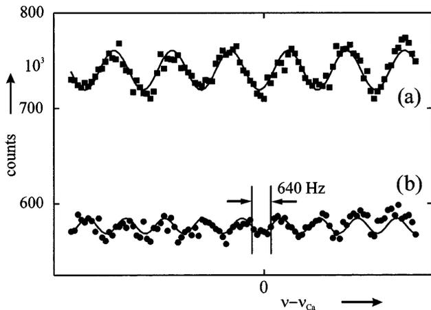
Fig. 4. Optical Ramsey fringes taken with slow Ca atoms for resolutions of 960 Hz (filled squares) and 640 Hz (filled circles) corresponding to pulse separations of  $T = 260 \mu\text{s}$  and  $T = 390 \mu\text{s}$  and fits (solid curves) according to relation (1).
